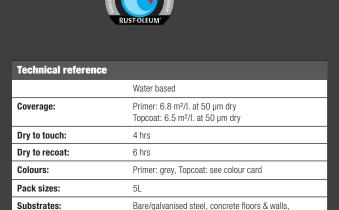
masonry, mineral fibre board.
